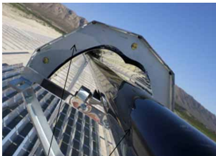
Figure 2.3: Receiver and Secondary Reflector Primary reflector (Source: Novatec)
