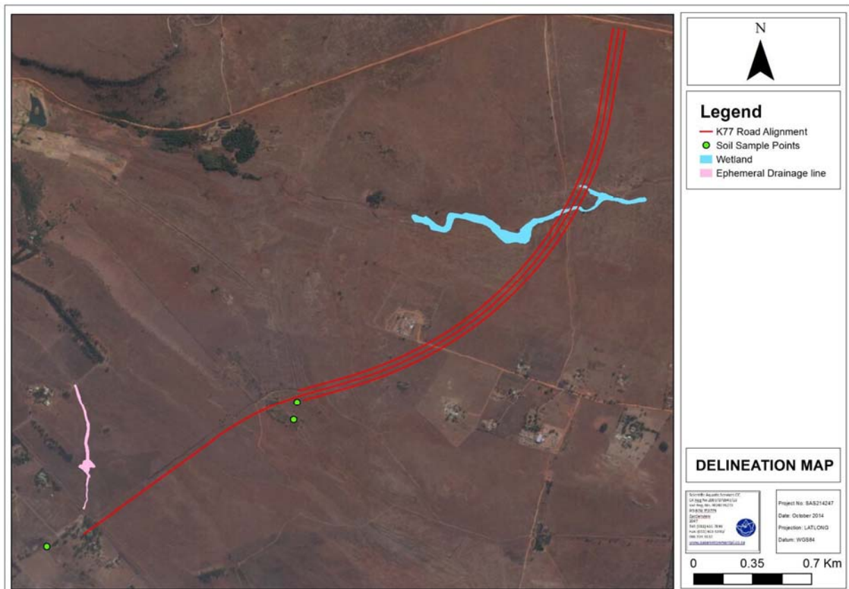
Figure 5: Drainage Features Along the K77 Route
