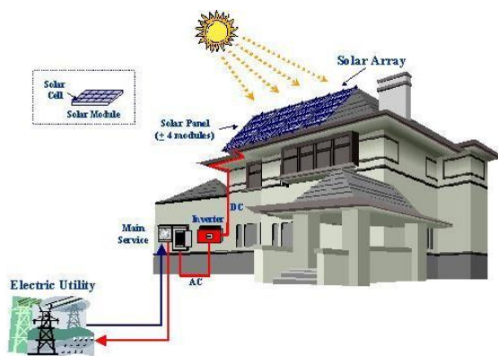
Figure 4: Energy flow between PV power generation facility with fixed modules and Electrical Utility
