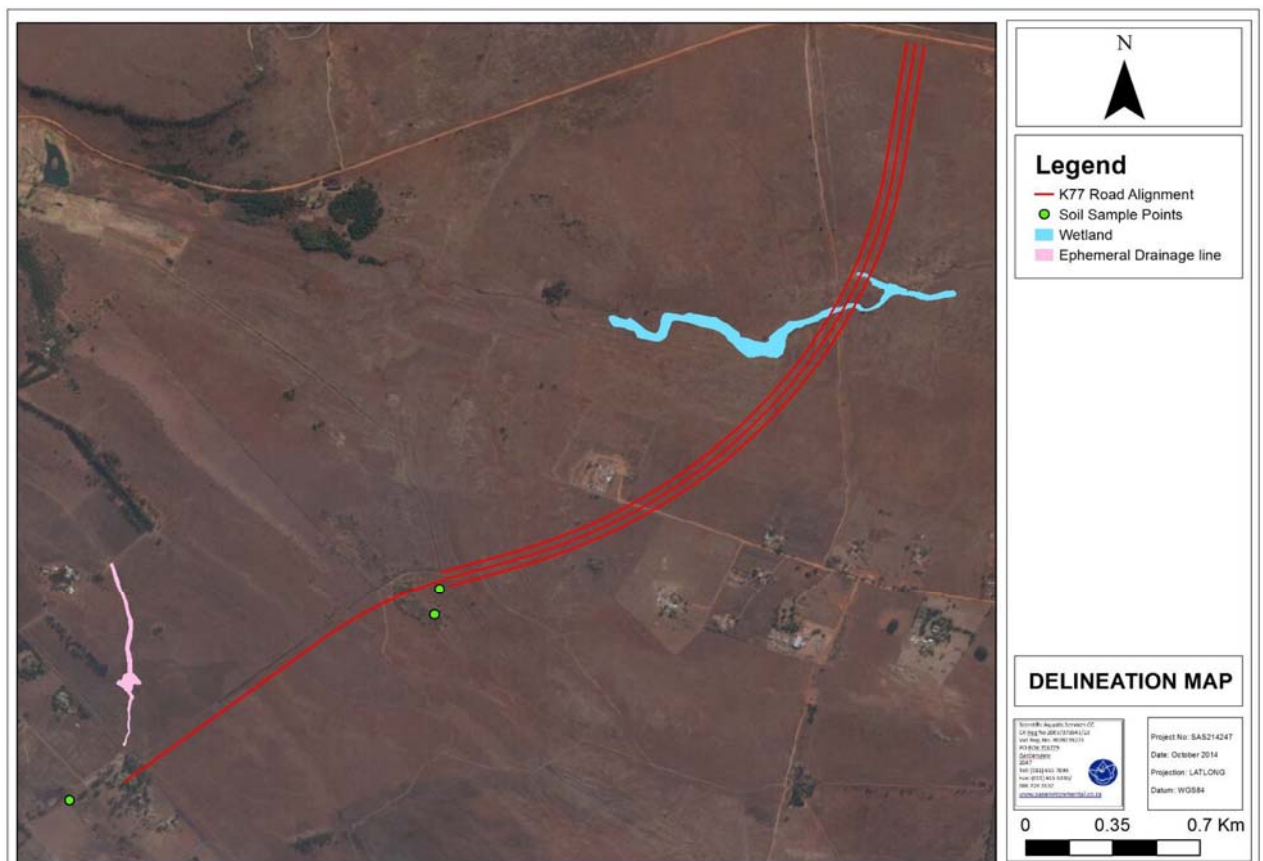
Figure 3: Drainage Features Along the K77 Route
