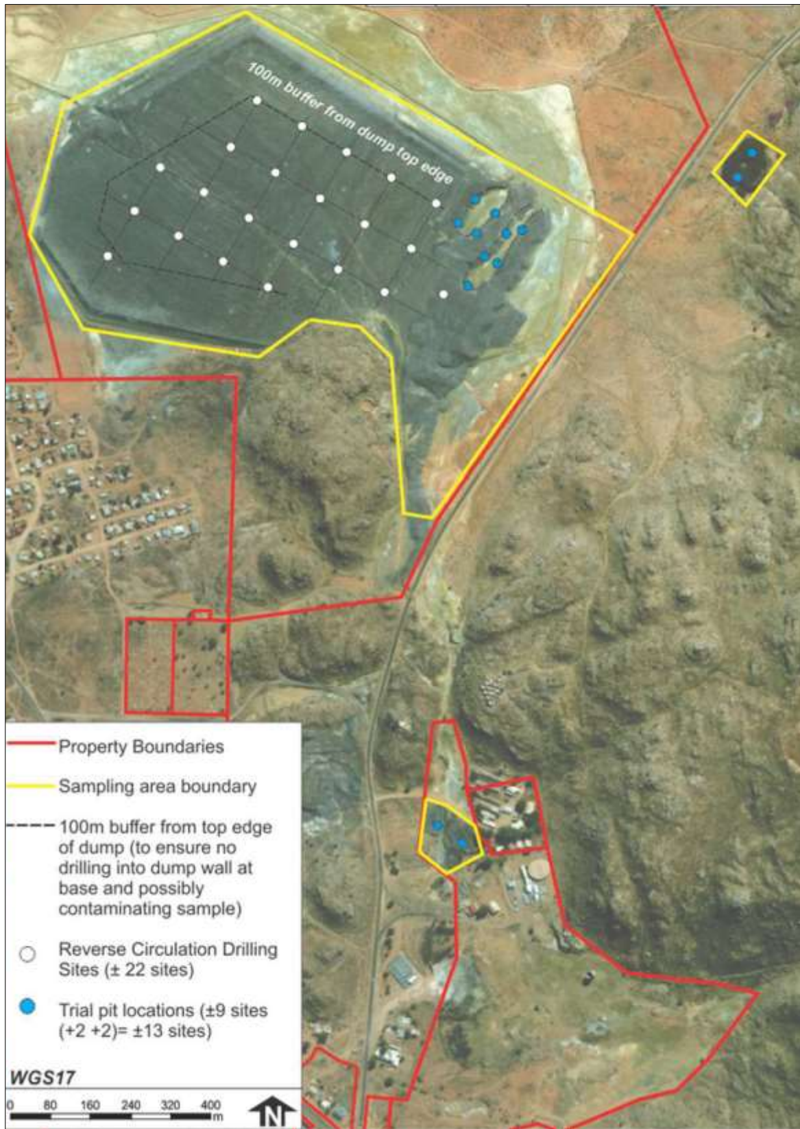
Figure 5. Detail locality of Okiep dumps under consideration, including site layout plan (Site Plan Consulting, May 2019)
