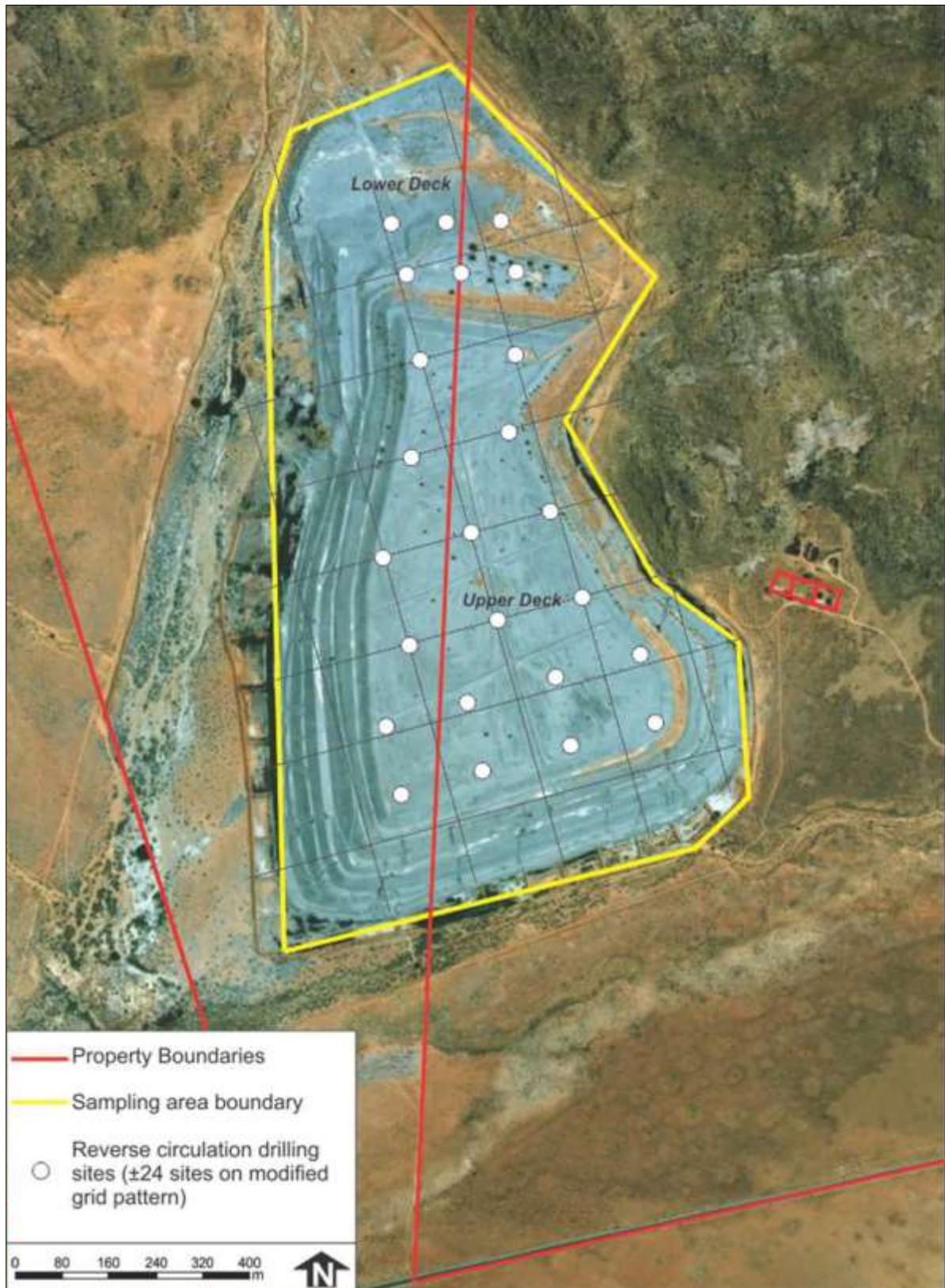
Figure 7. Detail locality of Carolusberg tailings dump including site layout plan (Site Plan Consulting, May 2019)
