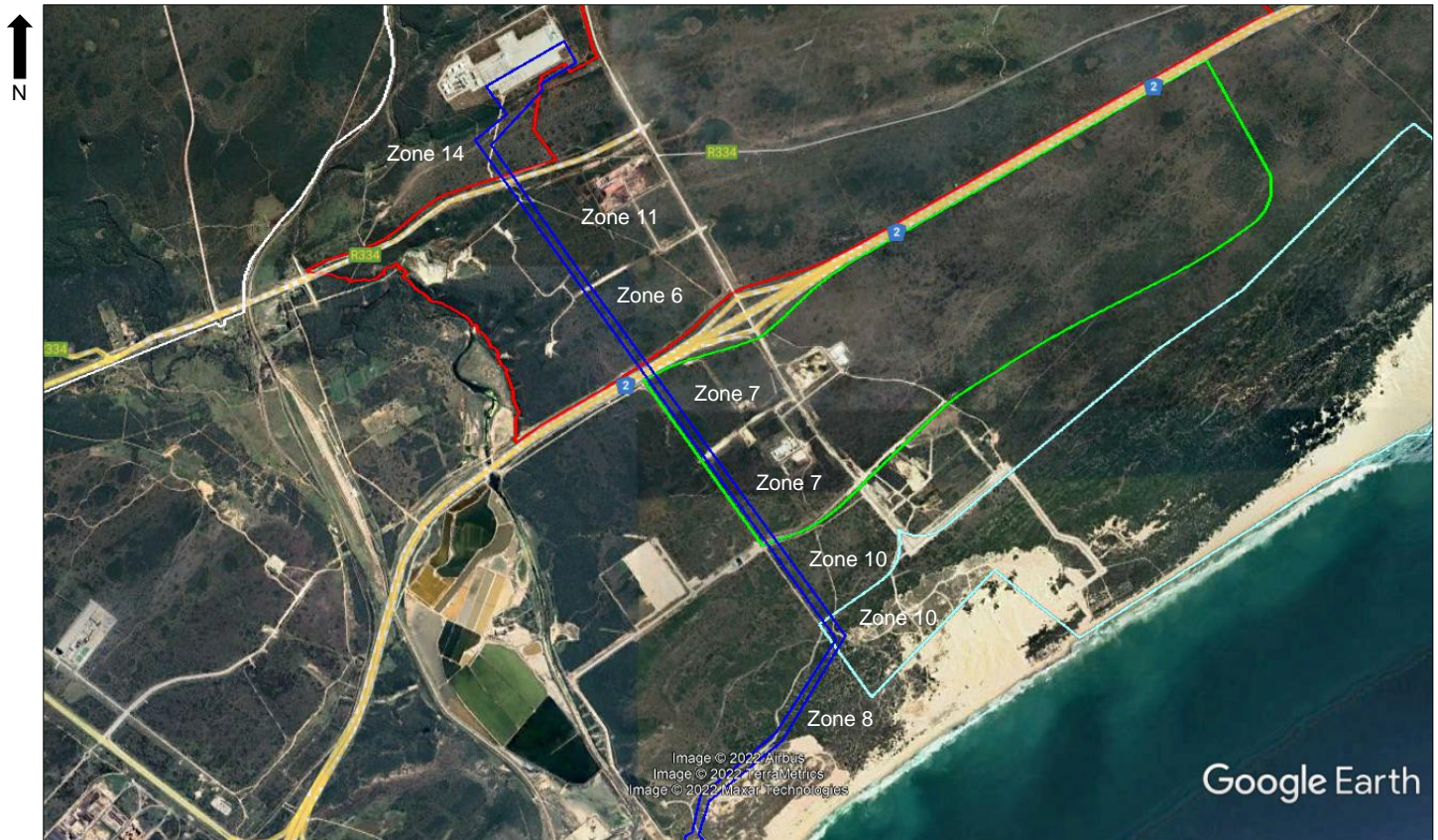
Figure 5. The preferred 132kV powerline route (dark blue line), crosses Zone 14, Zone 6, Zone 11 Zone 7, Zone 8 & Zone 10 in the Coega IDZ.
