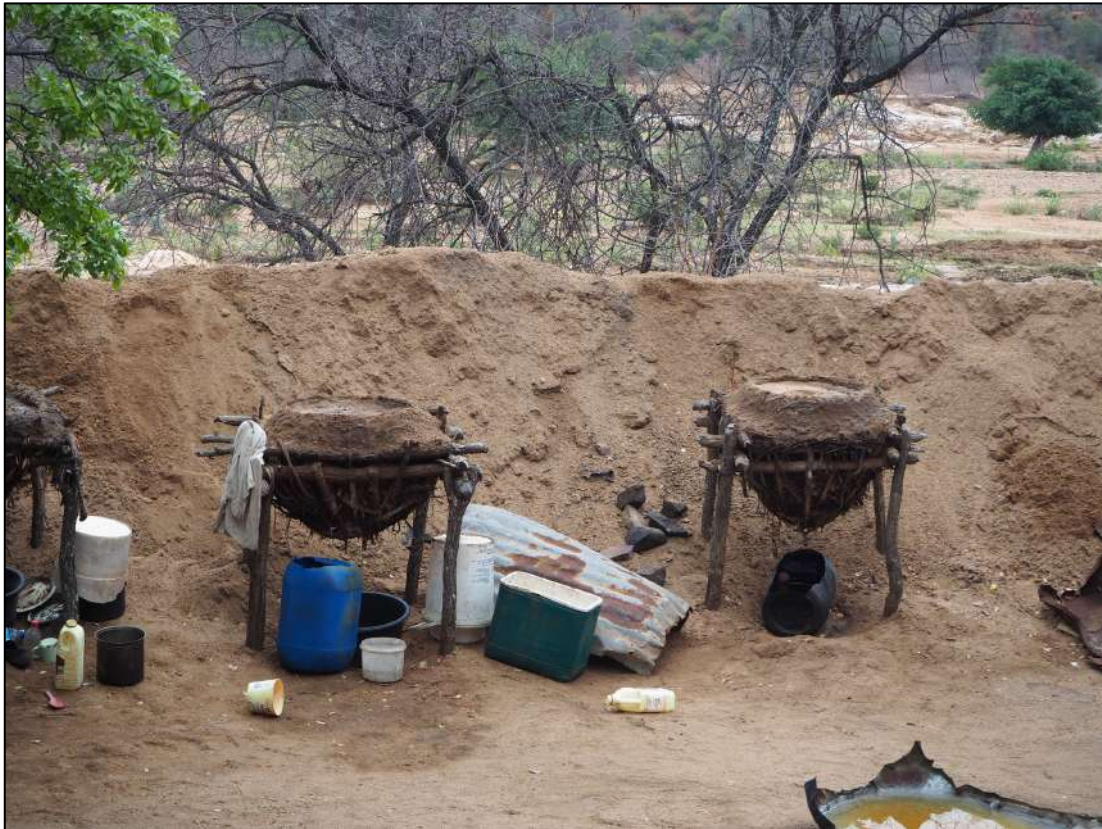
Figure 13. Mopane and Sand Filters
