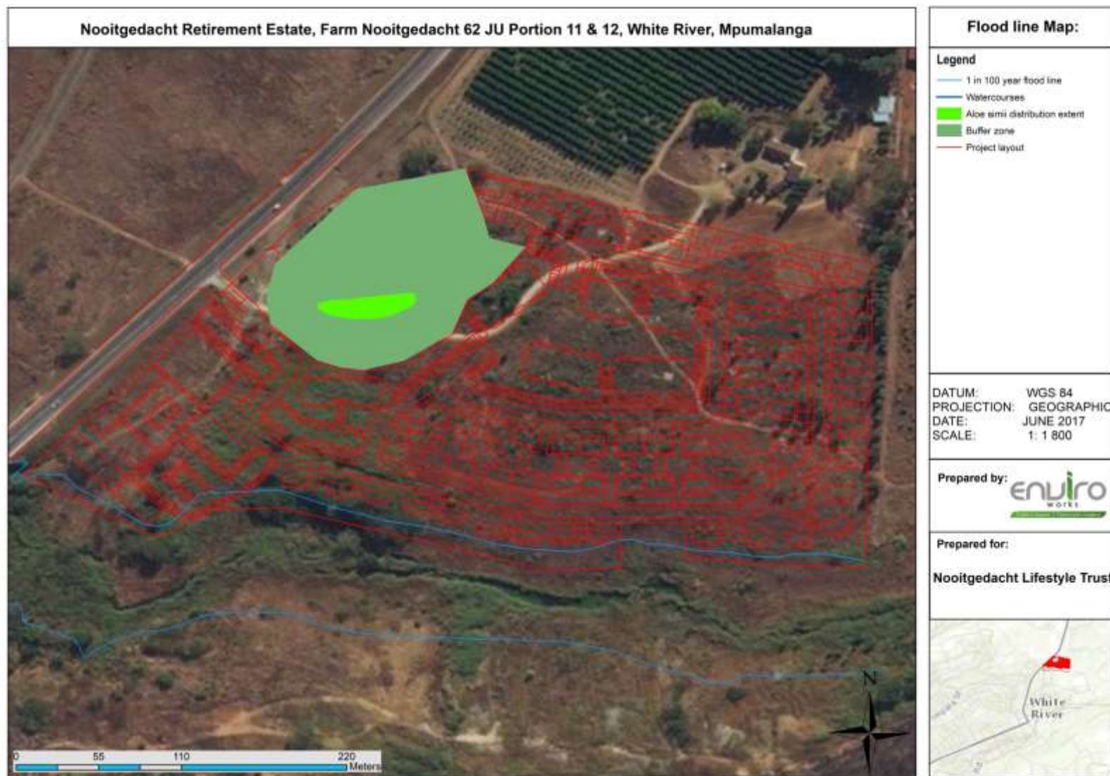
Figure 14: Flood line Map indicating the proposed buffer outside the 1:100 year flood line of the White River (see Appendix B for A 3 size)
