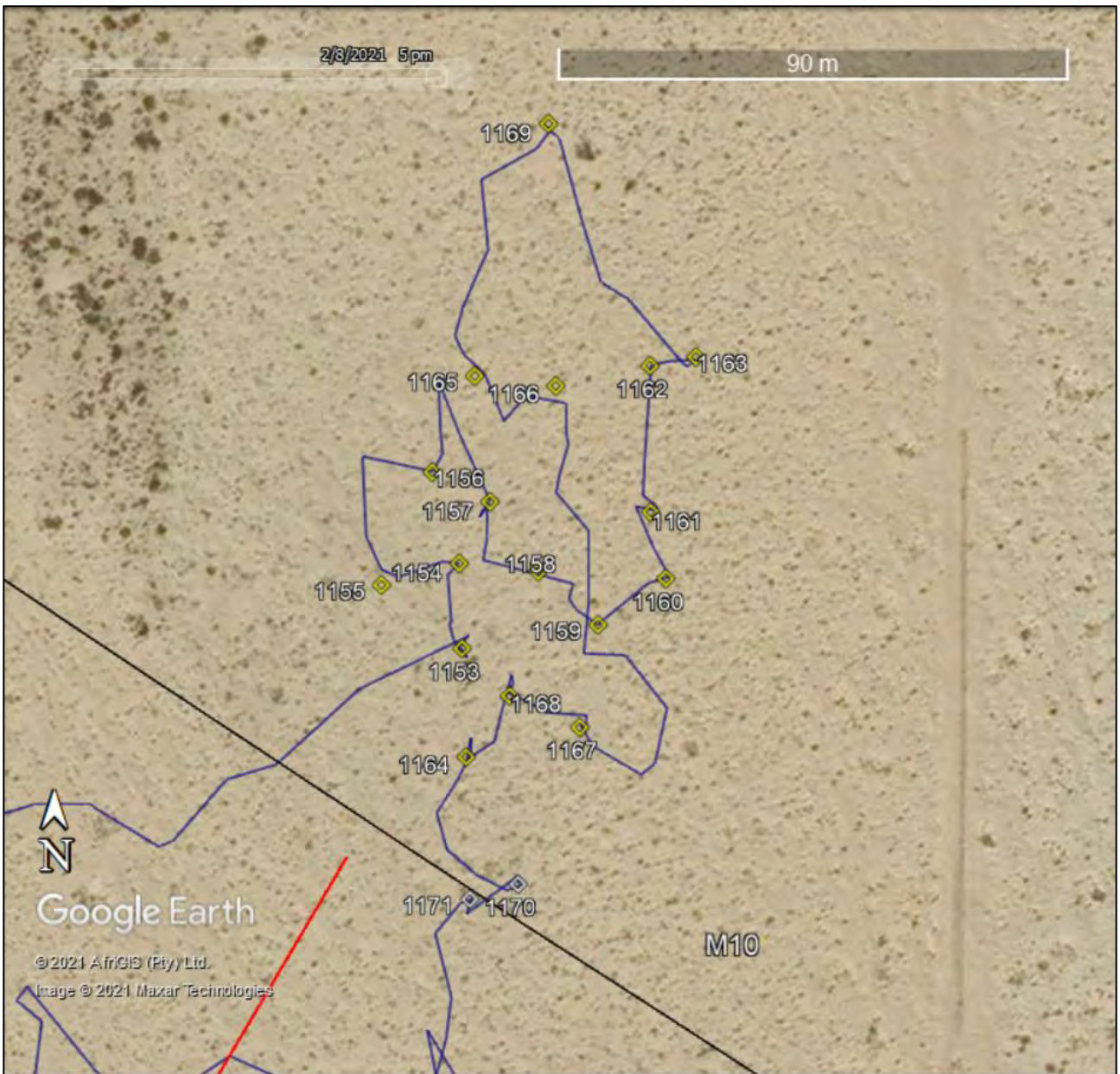
Figure A2.15: Detail Block M10. This site cluster lies on a dune crest just outside the block but would be in danger from slumping and deflation after excavation of the trench into the dune.
