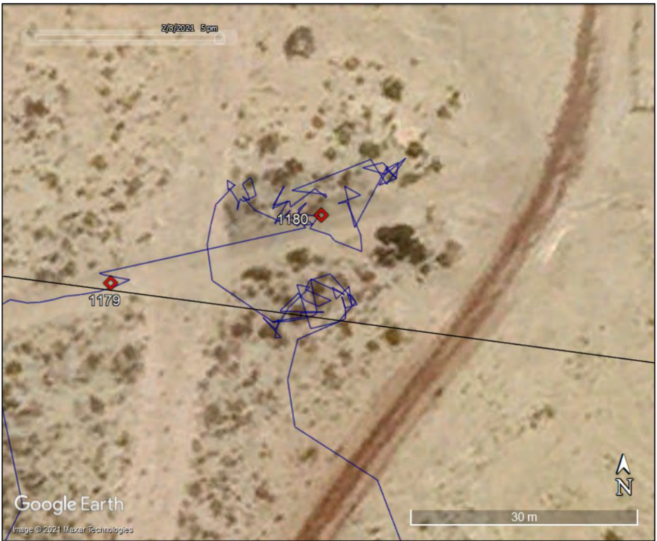
Figure A2.17: Detail Block M10. 1179 and 1180 fall in the Copper Railway and the dark patch around 1180 is the dump (material lies on both sides of the road). The brown road leads to the newly built oxidation ponds.
