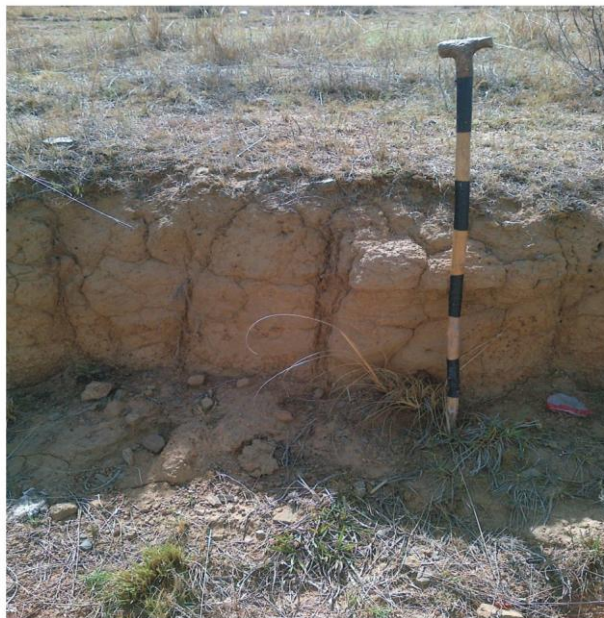
Figure 7. The terrain is capped by a thin mantle of grass-covered, Quaternary sediments (residual soils).
