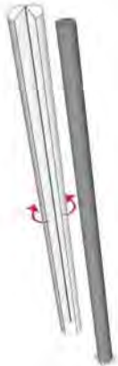
Step 4 mould removed from concrete
