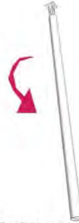
Step 3 The shutters are prepared and held vertically inverted and left to cure
