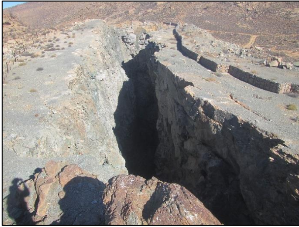
Figure 21: Deep excavation following a copper ore body at Carolusberg.
