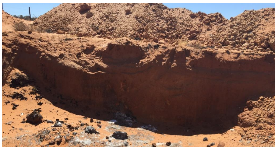
Plate 1: Prospecting pit (J028) showing depth (approximately 2 m) of the red aeolian sand. The white underlying kaolin surface is visible in the centre foreground
