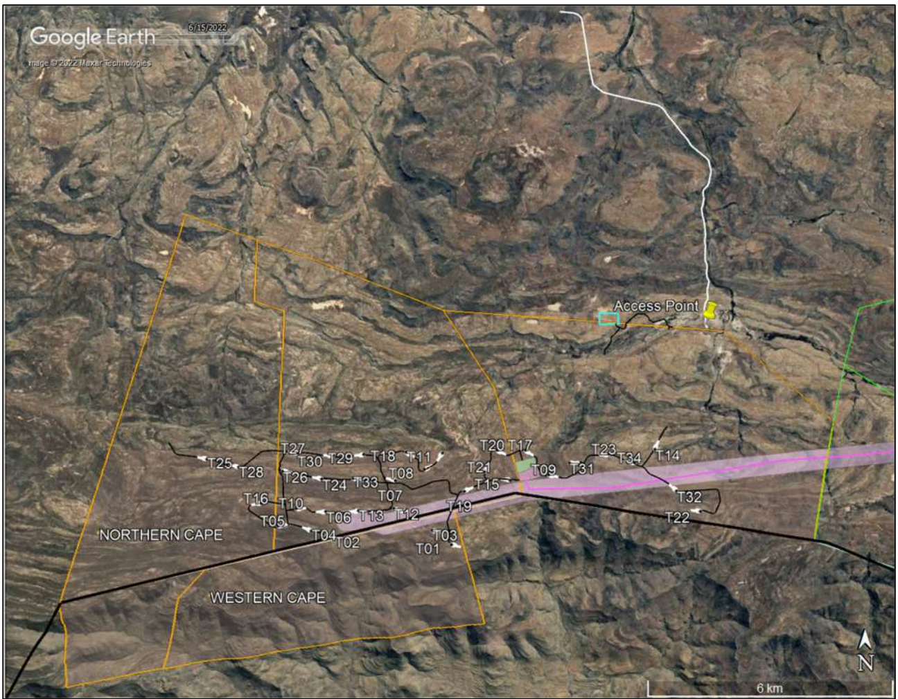
Figure 3: Aerial view of the study area showing the location of the project (turbine hardstands are white labelled stars, roads in black). Small, coloured polygons represent substations. Orange polygons are the affected properties and the access road is in white. The grid connection extends towards the east (pink) with its properties outlined in green.
