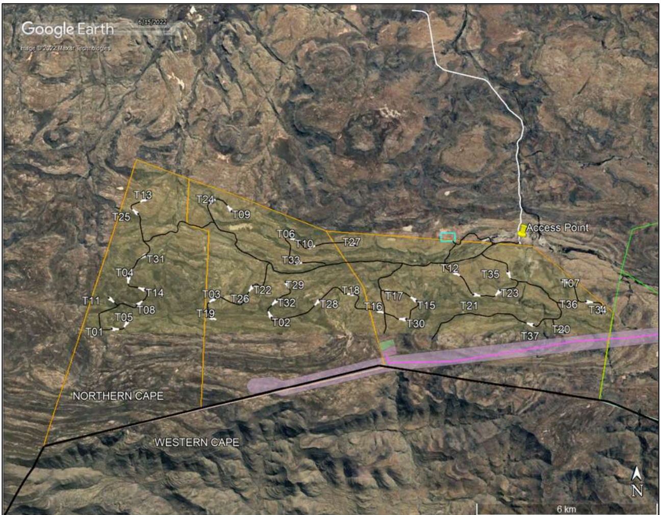
Figure 3: Aerial view of the study area showing the layout of the project (WEF farm portions = orange, grid farm portions = green, turbine hardstands = white labelled symbols, roads = black lines, main access road = white line, batching plant = green rectangle, on site substation = green [IPP portion] and pink [Eskom portion] square, 132 kV powerline = pink line within 500 m wide approved corridor).
