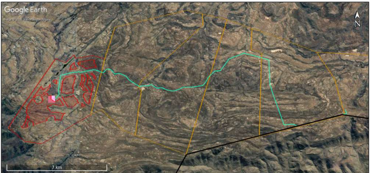
Figure 3: Aerial view of the study area showing the location of the project (red polygon = affected farm portion for the WEF, red shading = buildable area; pink square = Eskom substation, IPP substation, associated infrastructure and laydown area). The grid connection extends towards the east (turquoise line with farm portions outlined in orange). The black line is the provincial boundary with Western Cape.
