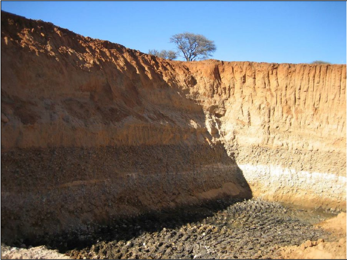
Figure 8: A diamond mining pit at Rietputs 15 showing hornfels bedrock overlaid by gravel and alluvial deposits. Source: Leader (2009: fig. 3.1).
