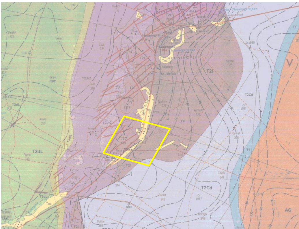
Figure 3: Geological map of the area around Farm Perth 343 indicated within the yellow rectangle. Abbreviations of the rock types are explained in Table 2. Map enlarged from the Geological Survey 1: 250 000 map 2622 Morokweng.
