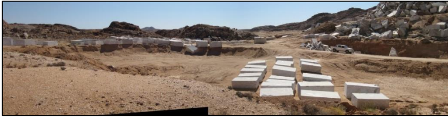
Plate 15: Granite blocks removed from the Central face lie in a borrow pit.
