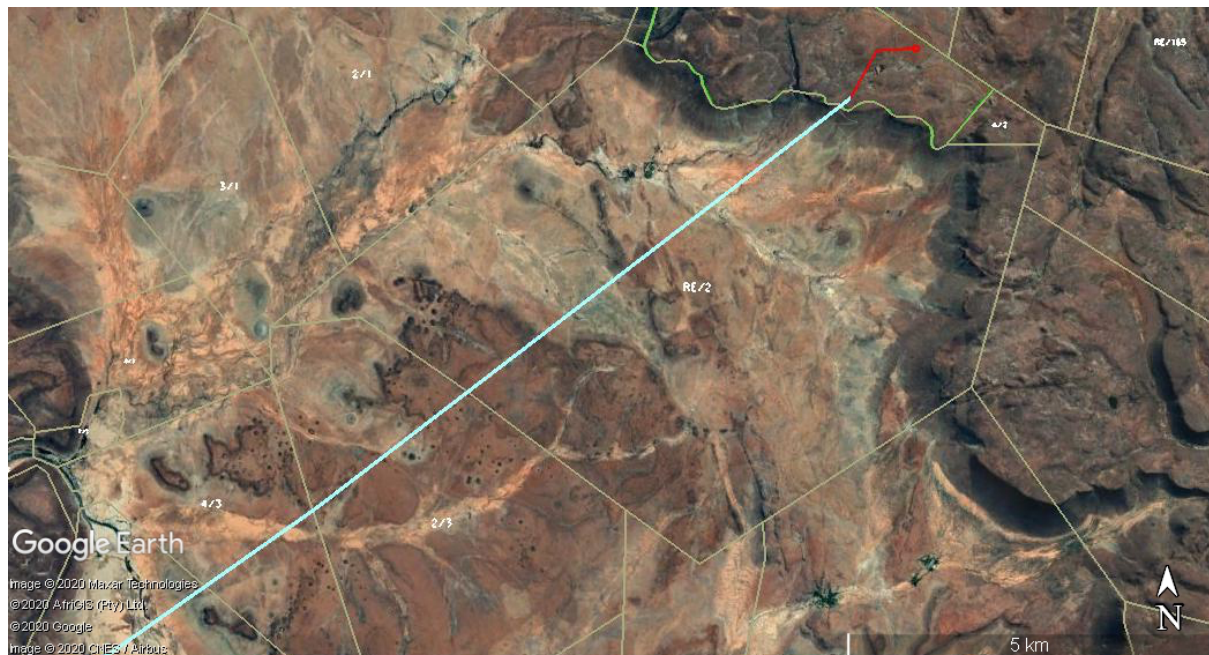
Figure 3: Google Earth map of the proposed routes for the Mulilo De Aar grid connection project. The routes near De Aar to connect PVs facilities are shown in blue lines with the red line showing a proposed new connection to a potential battery storage facility on the mountain top. (here called Route 1 north). De Aar is off the map to the southwest.
