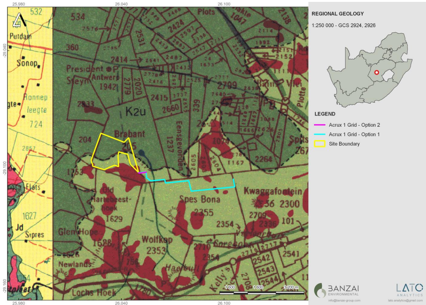
Figure 3. Extract of the 1:250 000 Bloemfontein 2926 Geological map (1966) (Council of Geoscience, Pretoria) indicating the geology of the Acruz Solar PV Project One and associated grid infrastructure near Bloemfontein in the Free State. The development is underlain by the Upper Stage of the Ecca Series (K2u), the Lower Stage (K3l) of the Beaufort System as well as dolerite in the south-east of the development.
