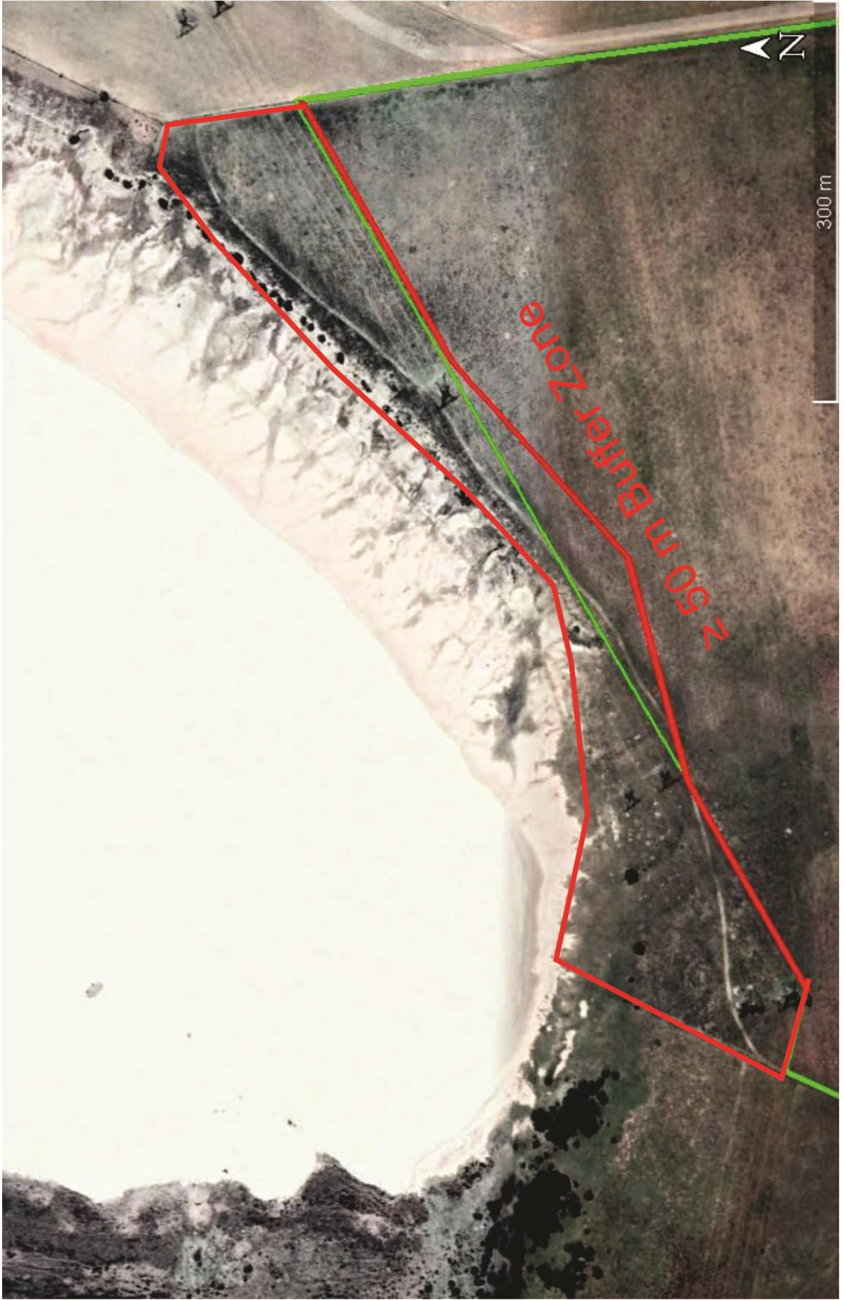
Figure 19. The pan dune deposits bordering the northern boundary of the site should be strictly avoided by a \geq 50 m no-go zone .
