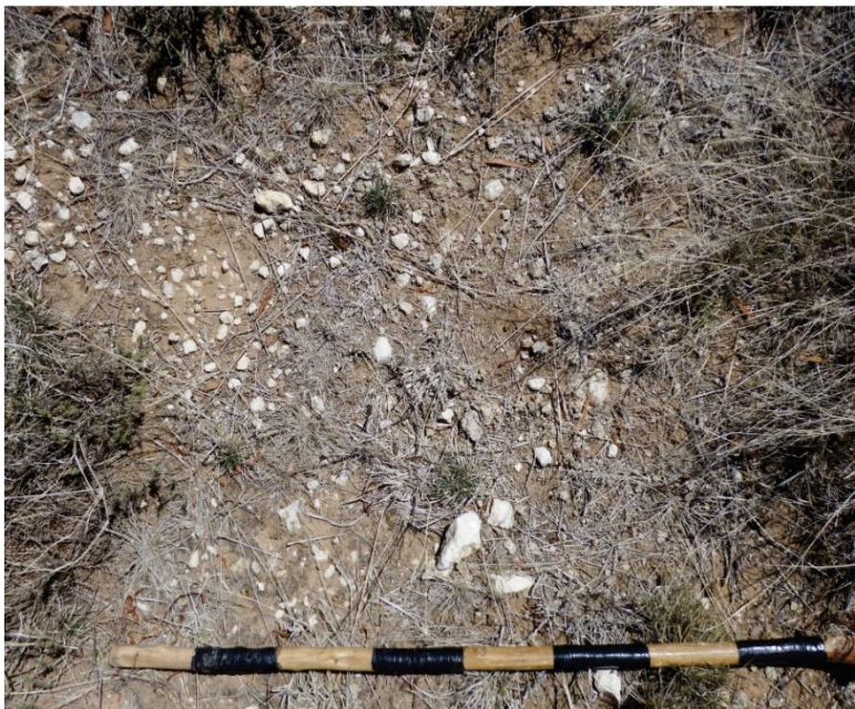
Figure 13. Tierberg Formation shale (above) covered by a well-developed and calcrete-rich aeolian sand overburden (below). Scale 1 = 10 cm
