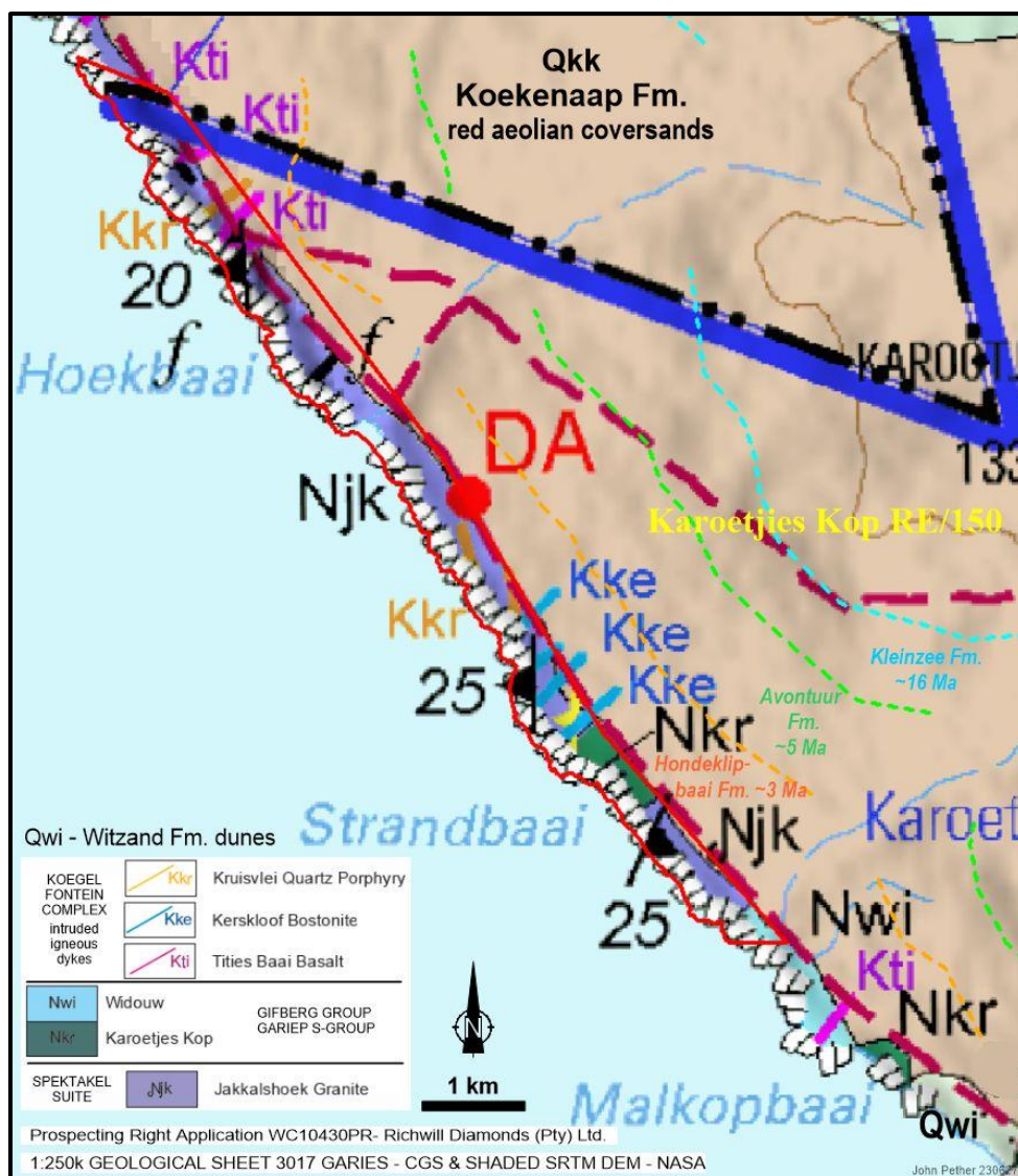
Figure 3. Surface geology of the Project Area and surrounds. The approximate subsurface extents of the underlying marine formations are also indicated.
