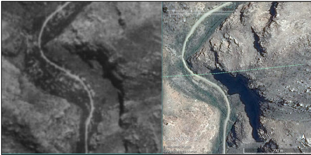
Figure 28: Comparative historical (1944; J Job 53, strip 8, photograph 2743) and modern aerial views of a section of the pass right in the middle of the Poort. The small borrow pits are more clearly evident in the earlier view as light patches.
