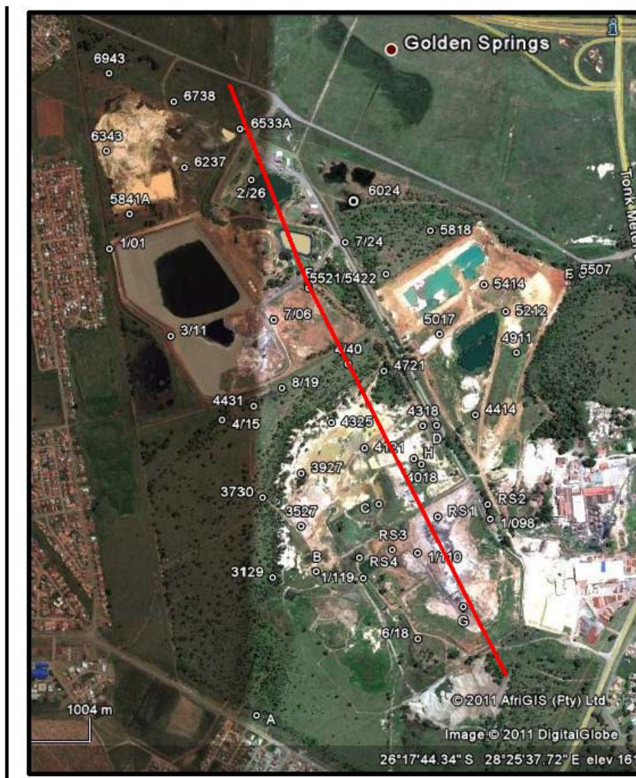
Figure 7-3: Borehole positions and location of dyke
