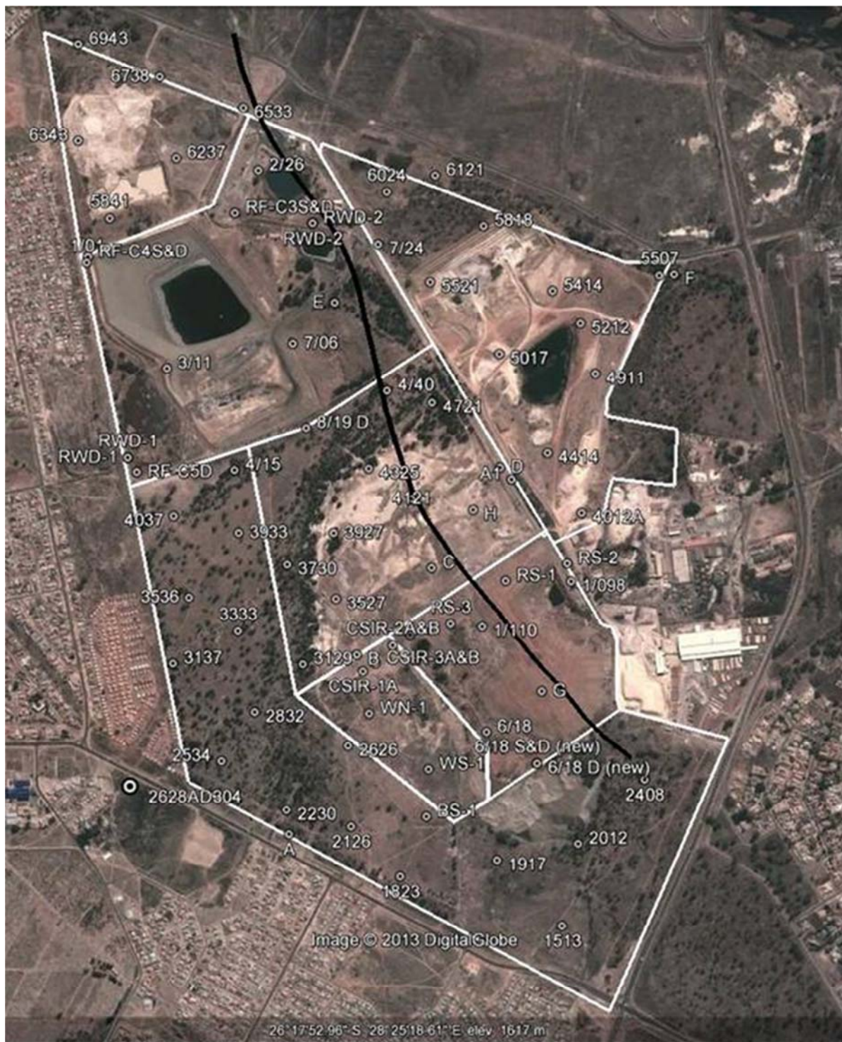
Figure 6-8: Locality map showing the positions of all boreholes drilled across the area investigated and also the position of the diabase dyke (black line) intruded into the formations. .
