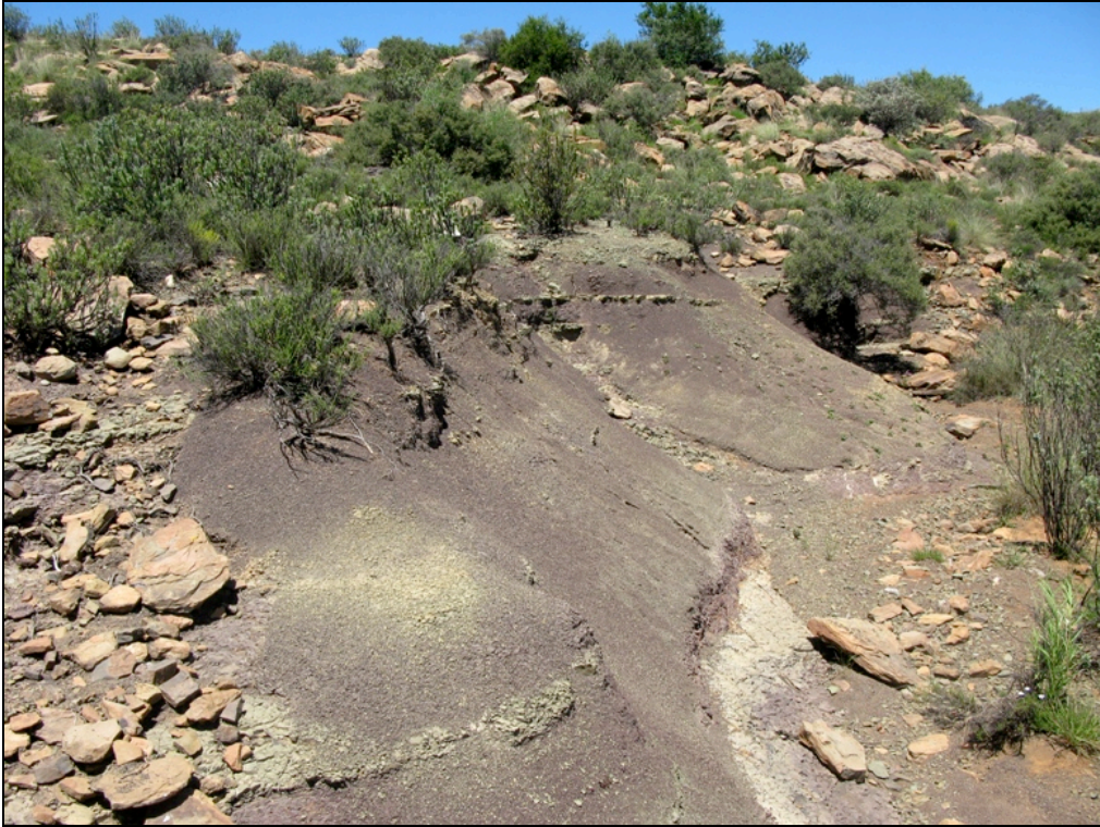
Fig. 3. Purplish-brown mudrocks and overlying channel sandstones (on the horizon) exposed on the south-eastern side of borrow pit site DR02404/8.5/0LR.
