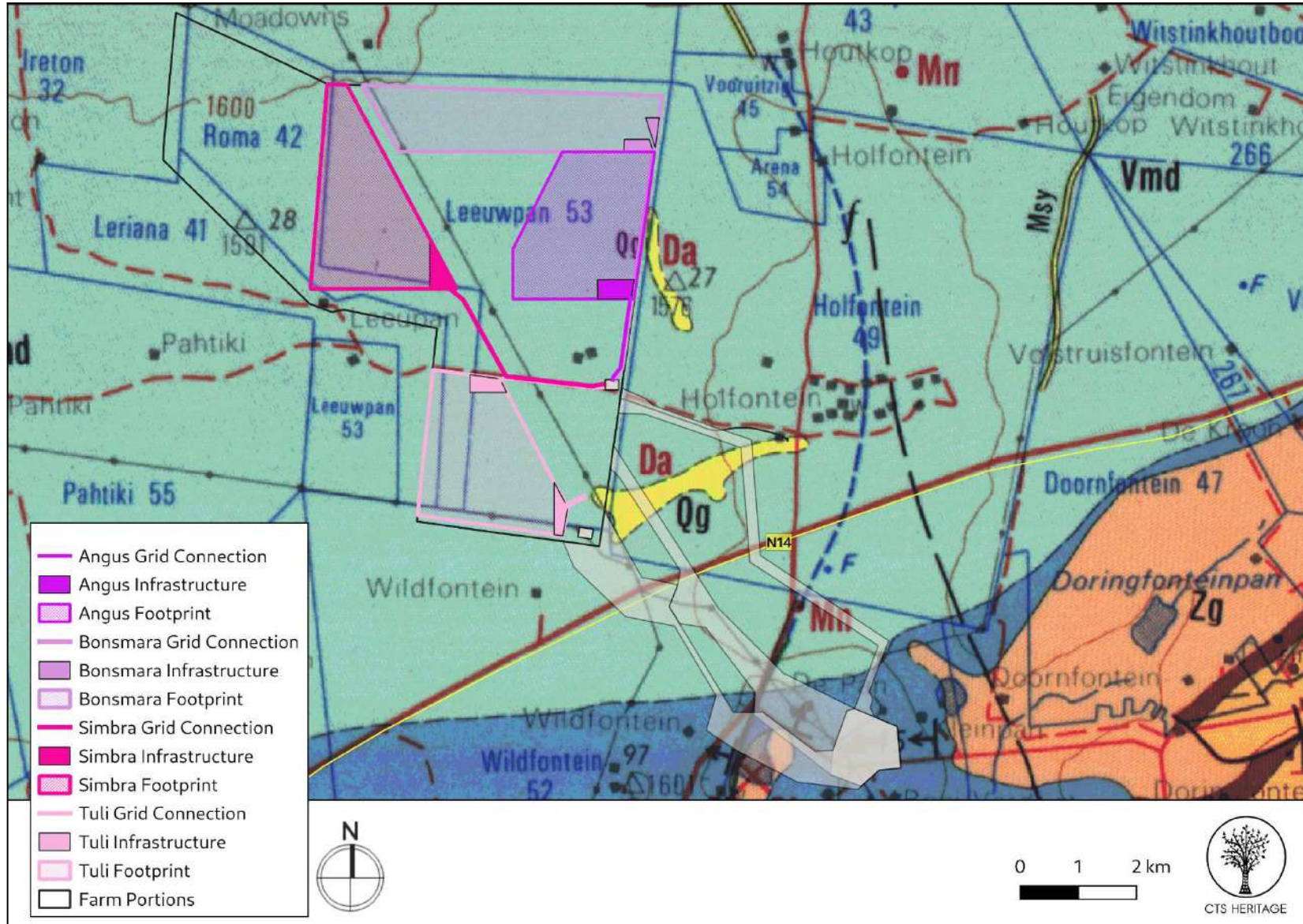
Figure 4.2. Geology Map. Extract from the CGS Map 2626 for West Rand indicating that the development area is underlain by Vmd: Malmani Subgroup sediments of the Chuniespoort Group
