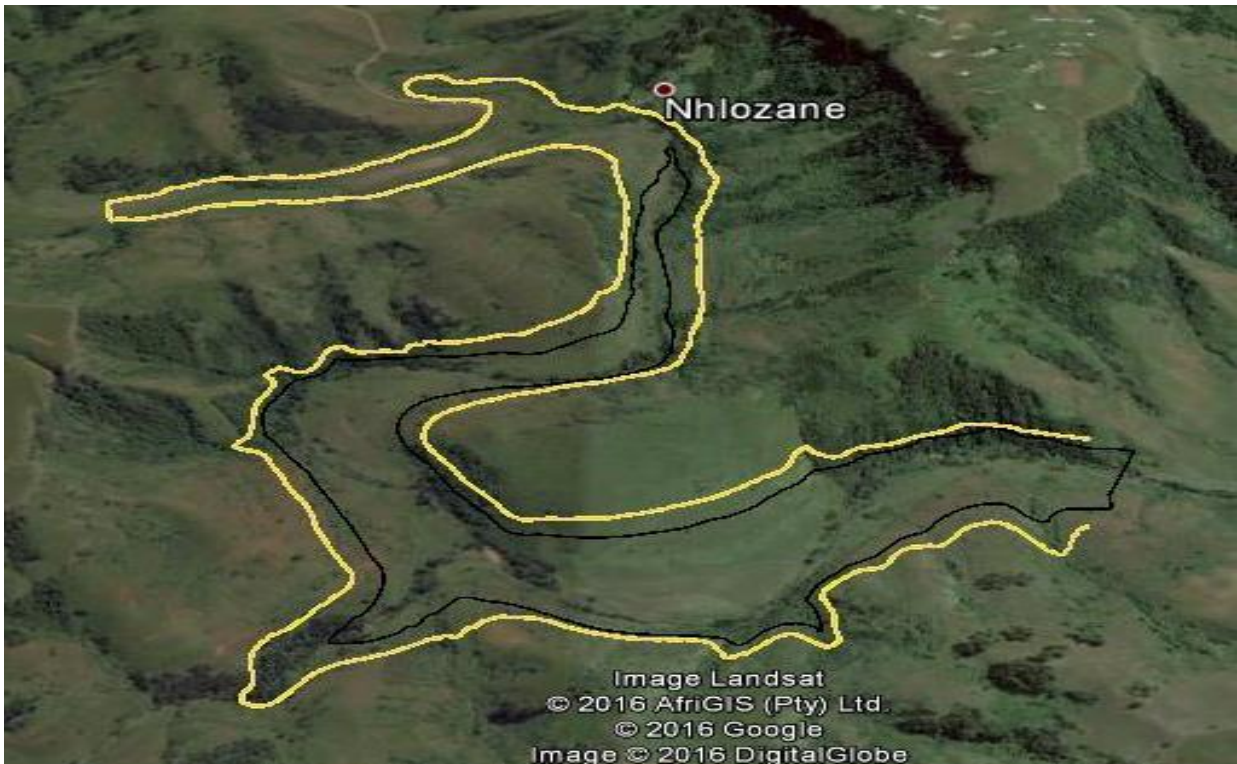
Figure 4: Google Earth image showing original and expanded inundation area of Dam Site 5
