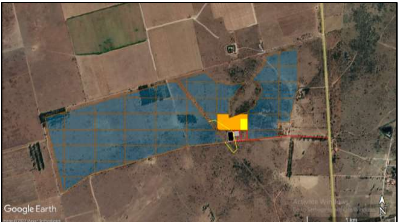
Figure 2: Google Earth Map of the proposed development of the Doornhoek 1 PV Facility with the sections shown by the orange outline. Blue sections are for the PV collectors, orange and yellow polygons are the amenities, with red lines for the grid connection.
