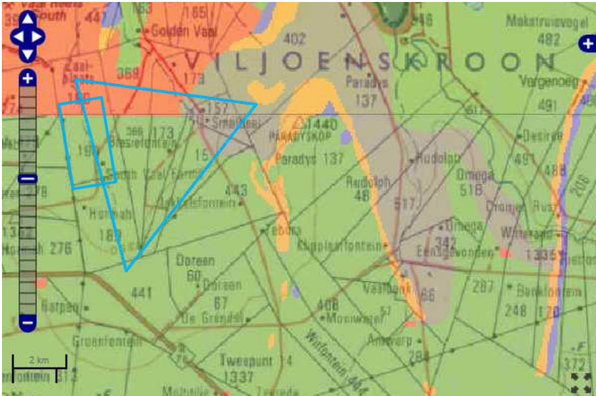
Figure 4: SAHRIS palaeosensitivity map for the site for the proposed Paradys PV Cluster shown within the blue polygon. Background colours indicate the following degrees of sensitivity: red = very highly sensitive; orange/yellow = high; green = moderate; blue = low; grey = insignificant/zero.
