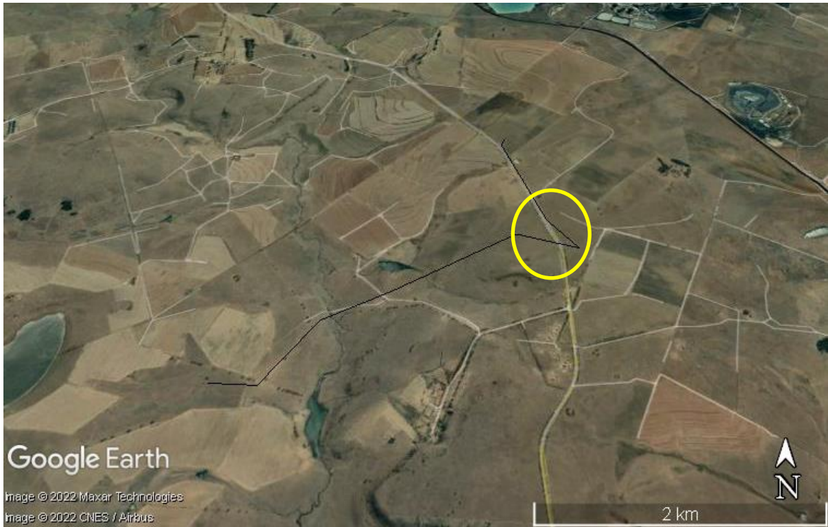
Figure 4: Grid Option 1 for Camden SEF (thin black line). Circle shows where the options differ.
