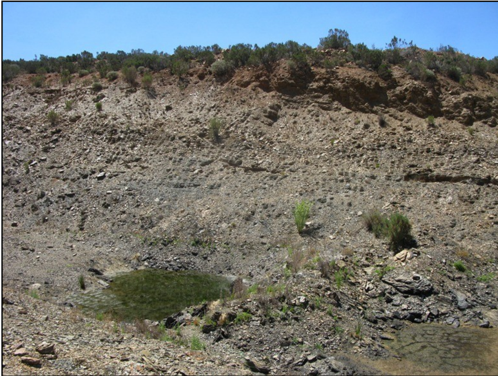
Fig. 4. Steep cut face through mudrocks and heterolithic beds within the upper Kweekvlei Formation in the NW portion of borrow pit DR01470/14.73/L/50/A/C33.
