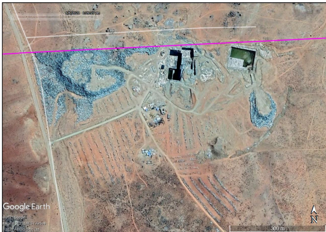
Figure 24: Example of a granite mine immediately inside the northern boundary of the study area showing the landscape scarring created by mining, mine dumps and stockpiling of product.
