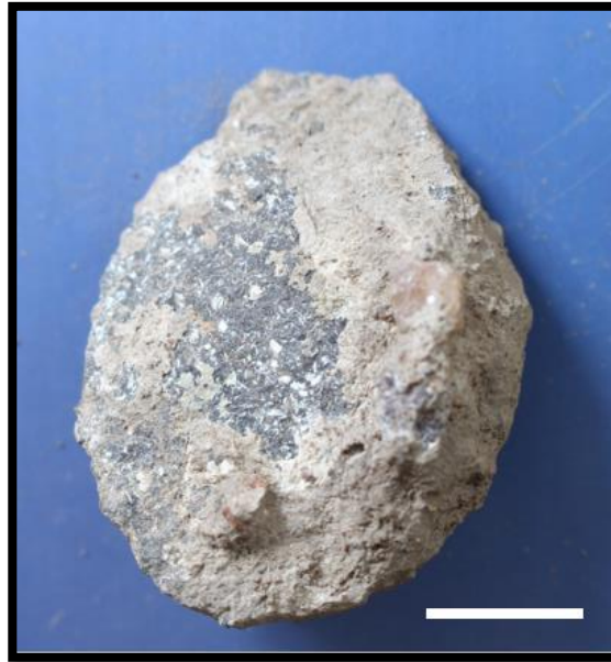
Figure 4.4: No. 1241 shows the medium-grained texture of OBP dolerite samples and fine plagioclase laths. This sample is coated in calcium carbonate. The white bar represents 1 cm. Ex situ dolerite around OBP is aphanitic and has a brown weathered surface and a black, fresh surface (OBP 4G; OBP 5A, D and, E). Plagioclase laths are only visible in OBP 5D (~10%).
