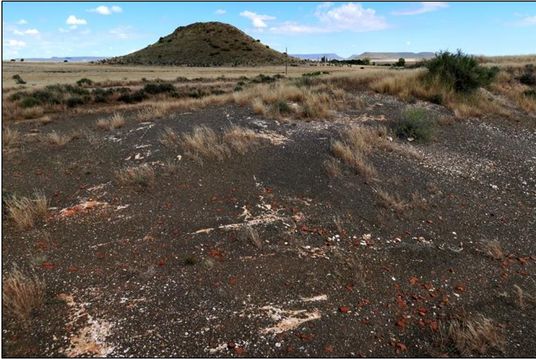
Figure 12: Dark grey, weathered, crumbly Tierberg Formation mudrocks with extensive secondary calcrete veination (probably Quaternary age) exposed in roadside borrow pit excavation on Farm Wolwe Kuilen 1/42, just north of Wolwekuil farmstead on Farm Wolwe Kuilen RE/42.
