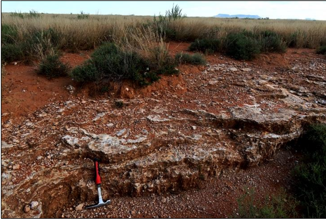
Figure 22: Heavily calcretised, orange-brown cover sands overlying weathered Tierberg Formation bedrocks on the margins of a borrow pit on Farm Wolwe Kuilen 1/42, just north of Wolwekuil farmstead on Farm Wolwe Kuilen RE/42 (See Figure 12) (hammer = 30 cm).
