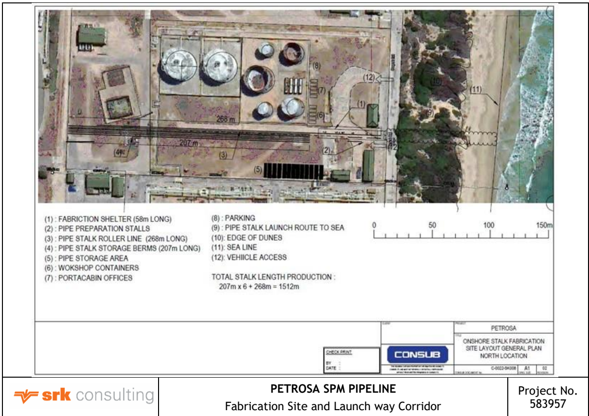
Figure 1-3: Fabrication site and launch way corridor
