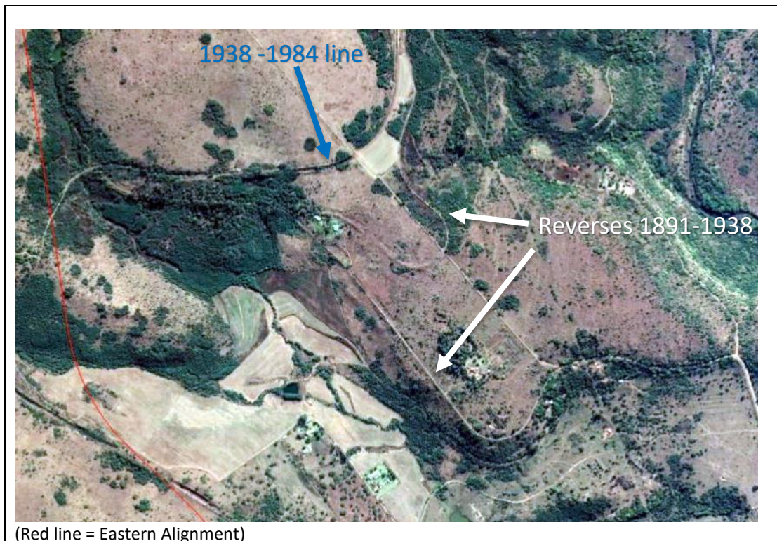
Figure 14. Track-beds of the old railway – line and reverses still to be seen in the landscape (Image: Google Earth)
