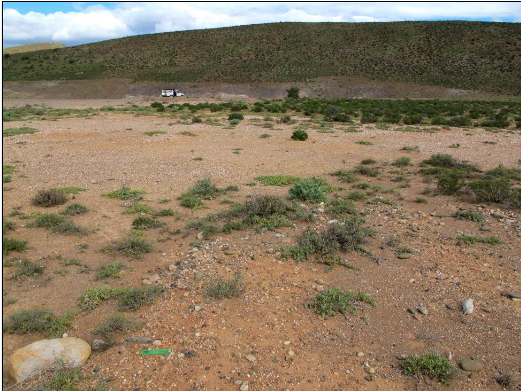
Figure 6: View towards the south of the existing pit showing the coarse alluvial gravels in the foreground and the over-lying veneer of fine silty alluvium with finer quartz clasts in the middle ground. The green ruler in the bottom left corner of the image is about 15cm in length.
