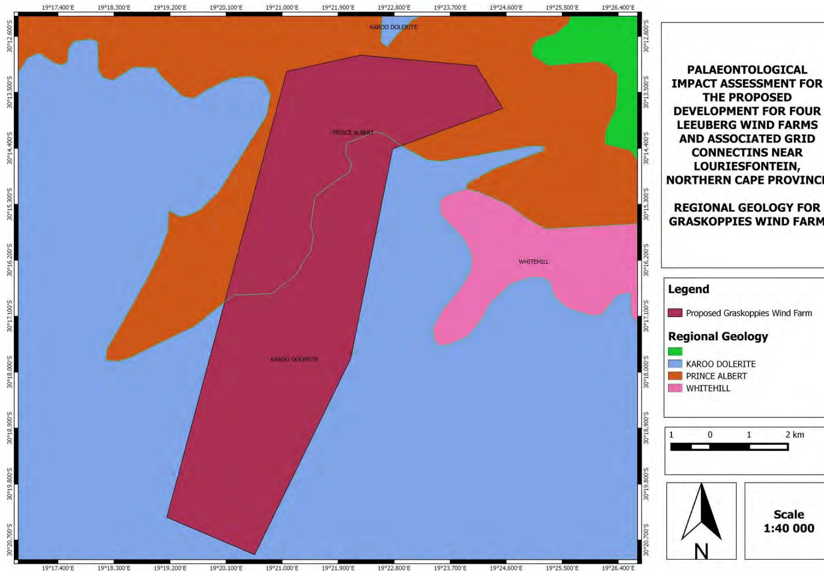
Figure 6: The surface geology of the proposed Graskoppies Wind Farm near Loeriesfontein in the Northern Cape Province. The development footprint is underlain by Karoo Dolerite as well as the Prince Albert and Whitehill Formations of the Ecca Group.
