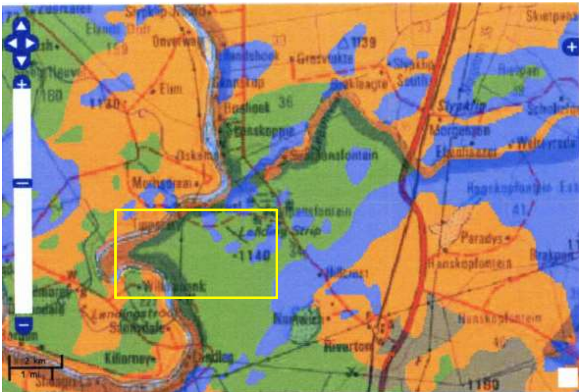
Figure 3: SAHRIS palaeosensitivity map for the site for the proposed prospecting and mining rights application on Farm Zoutspanfontein 34 shown within the yellow rectangle. Background colours indicate the following degrees of sensitivity: red = very highly sensitive; orange/yellow = high; green = moderate; blue = low; grey = insignificant/zero.
