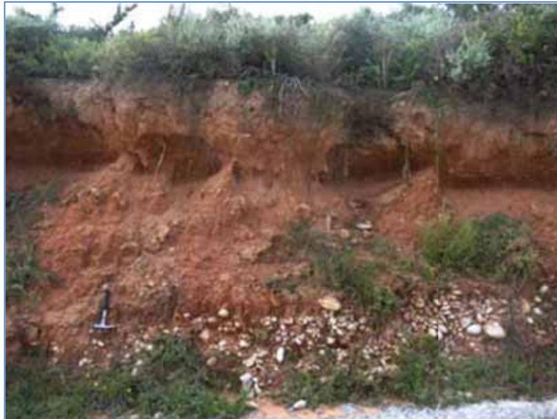
Figure 14B.8: Thick reddish-brown silty alluvium overlying fluvial pebbly and cobbly conglomerates exposed in a Zone 9 road cutting to the northeast of the marshalling yard (Hammer = 29 cm). The upper alluvial sediments here are partially calcretised around plant roots.
