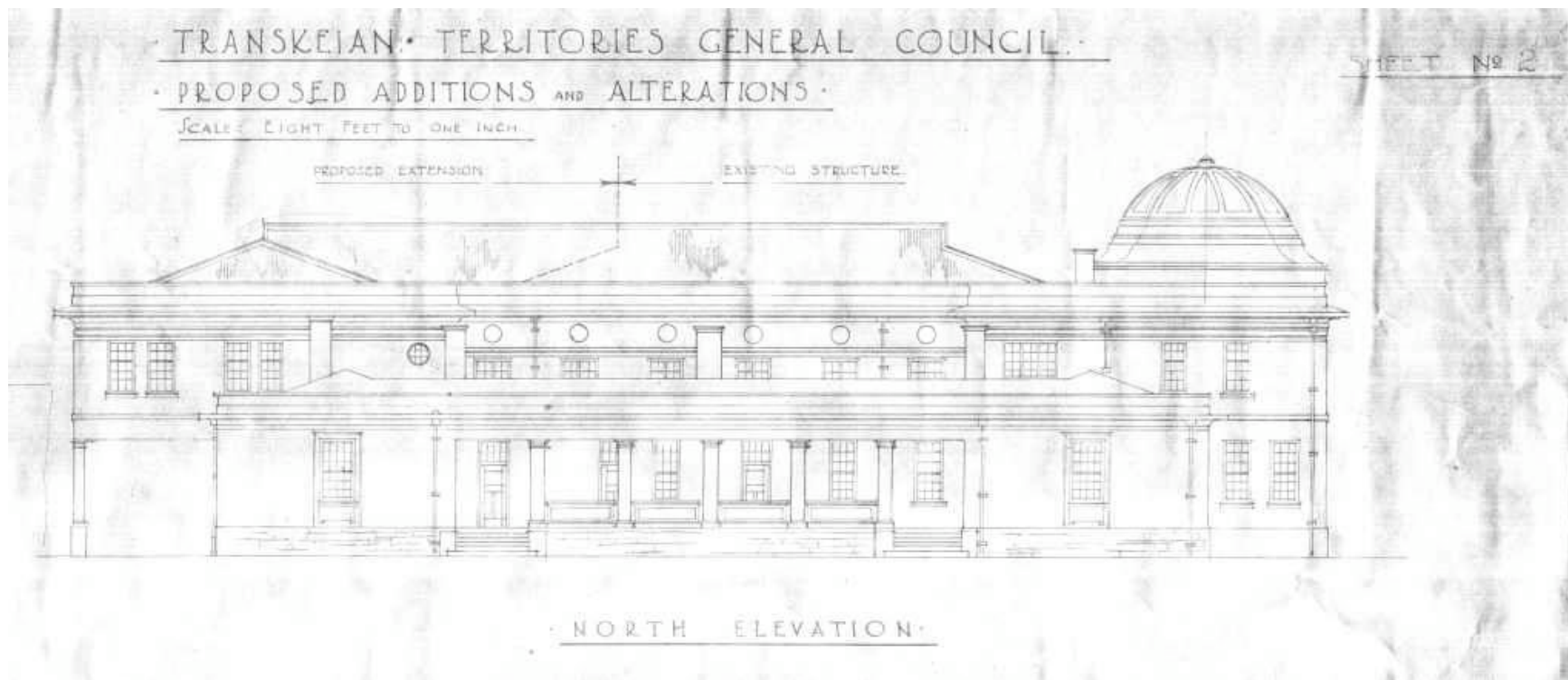
North Elevation of the Bhunga Building showing the proposed first floor extension on the left hand side. Office of the Engineer, UTTGC, Umtata, Extract from Sheet 2 of 2, Cape Archives M3/4046
