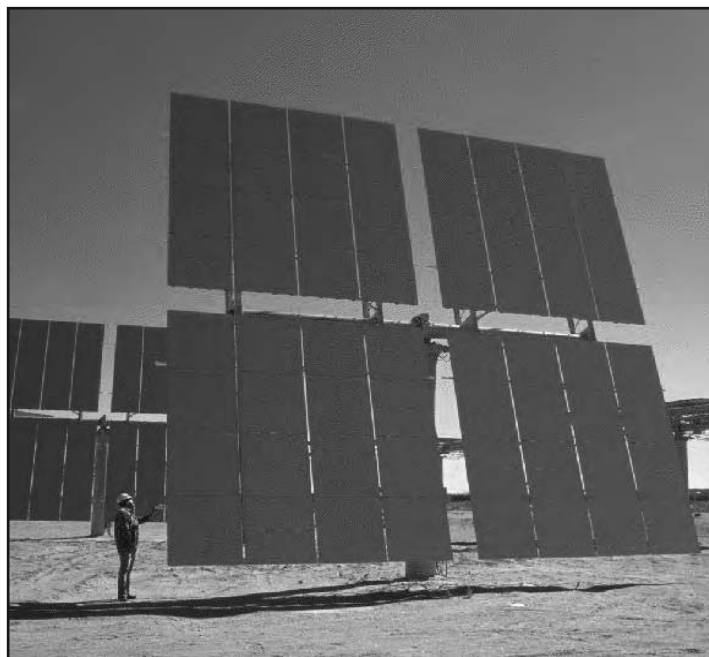
Figure 4- Single heliostat – image courtesy NREL
