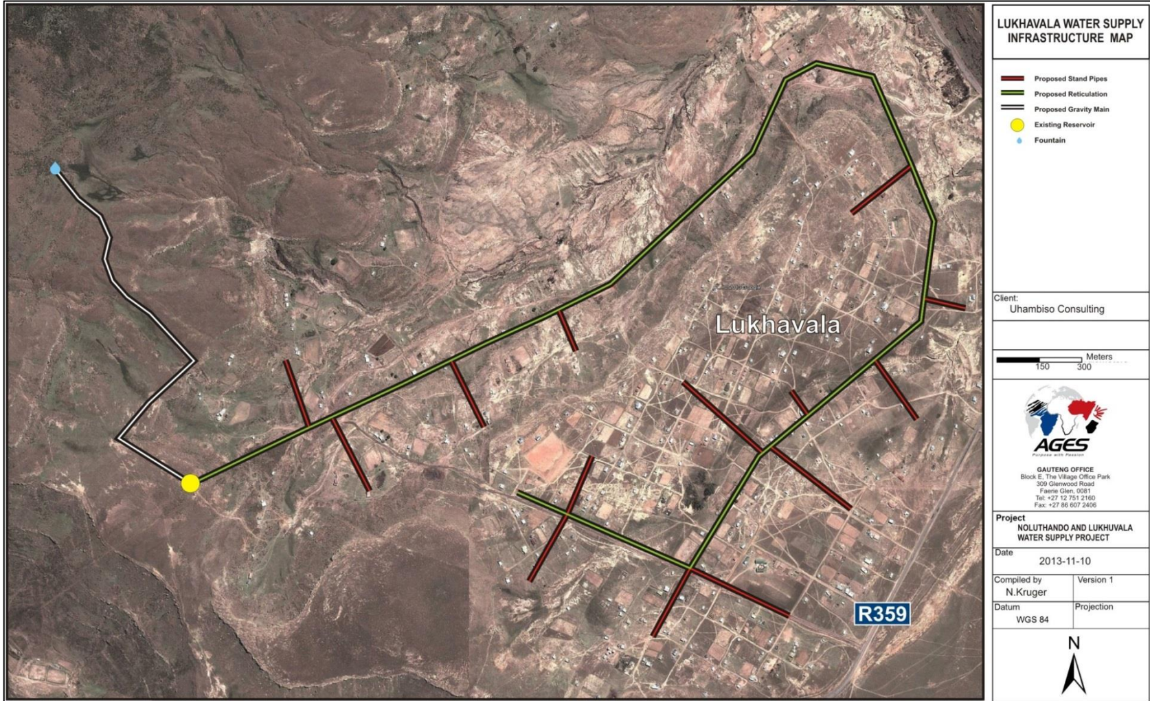
Figure 2-6: Aerial imagery indicating a regional context and infrastructure alignments in Lukhavala for Lukhavala and Noluthando Water Supply Project.
