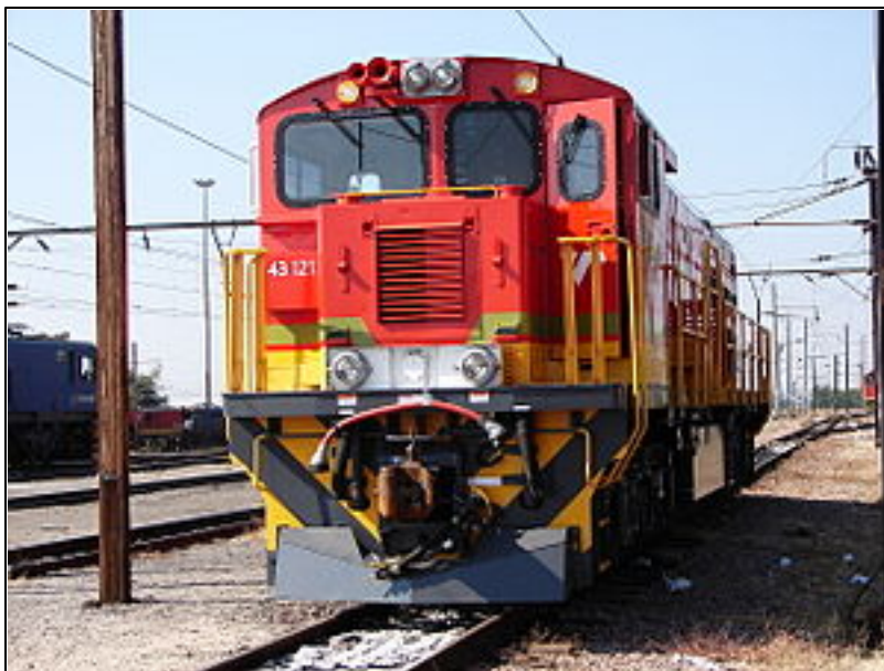
Figure 4-2: Class 43 diesel locomotives
