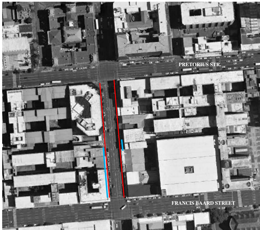
Fig. 75 Google Earth (2009) image of block 5 with positions of granite kerbing (red) highlighted.
