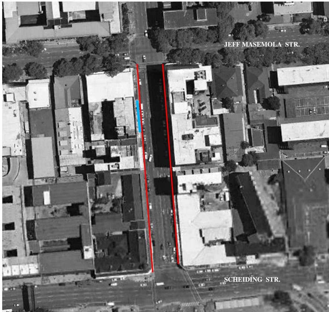
Fig. 161 Google Earth (2009) image of Block 10 with position of slate paving (blue) and granite kerbing (red) highlighted.
