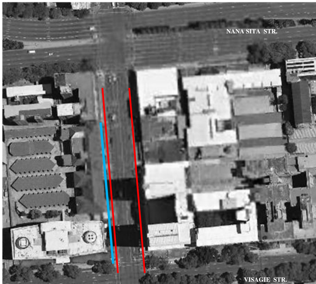
Fig. 99 Google Earth (2009) image of block 7 with position of slate paving (blue) and granite kerbing (red) highlighted.
