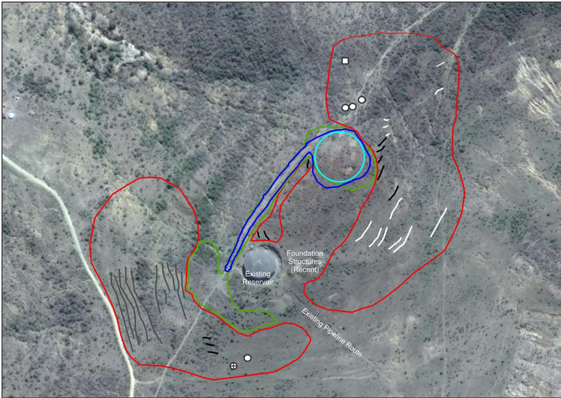
Figure 3: Aerial view indicating the locations of infrastructure, impact footprints, exciting surface features as well as heritage features and sensitive areas at the site of the Sandile Water Treatment Works Reservoir.
