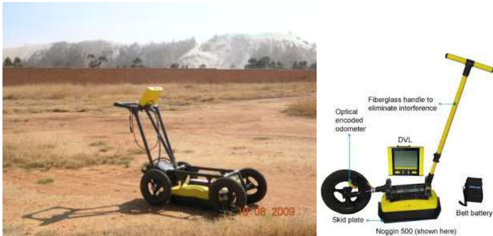
Figure 5: The Rock Noggin Smart Cart 250 MHz system (left) and a 500 MHz system (right)
