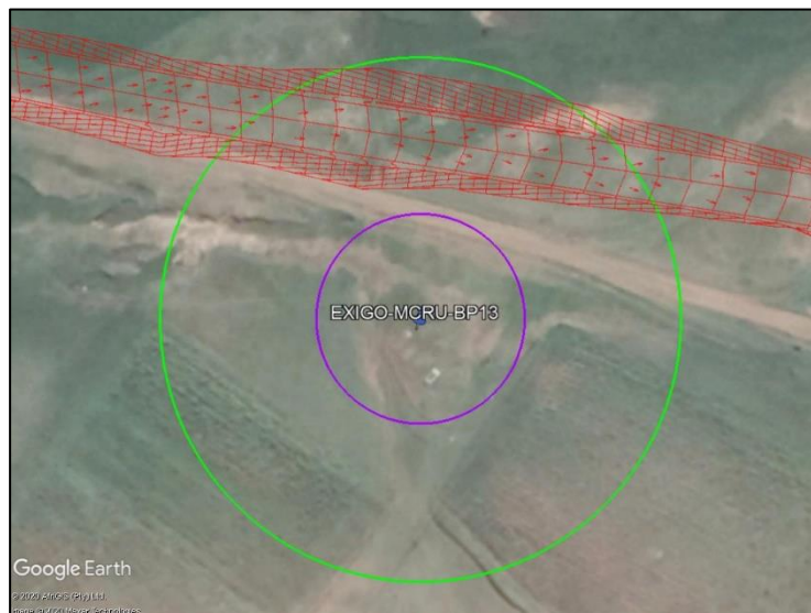
Figure 5-59: Site EXIGO-MCRU-BP13 with 20m buffers (purple) and 50m buffer (green) indicated in relation to the road design (red lines).
