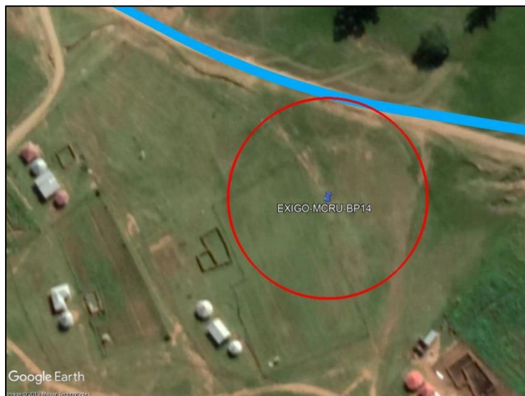
Figure 5-61: Site EXIGO-MCRU-BP14 and a required 50m conservation buffer (red line) in relation to the road alignment (blue line).
