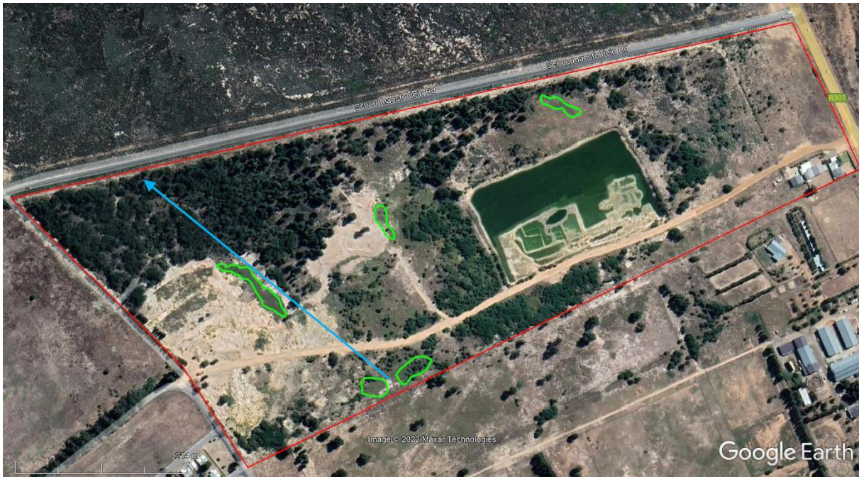
Figure 26: Google Earth image showing the delineated wetlands within the proposed development site. The remaining subsurface path detectable in past aerial images and still contains associated wetland habitat is indicated by the blue arrow.
