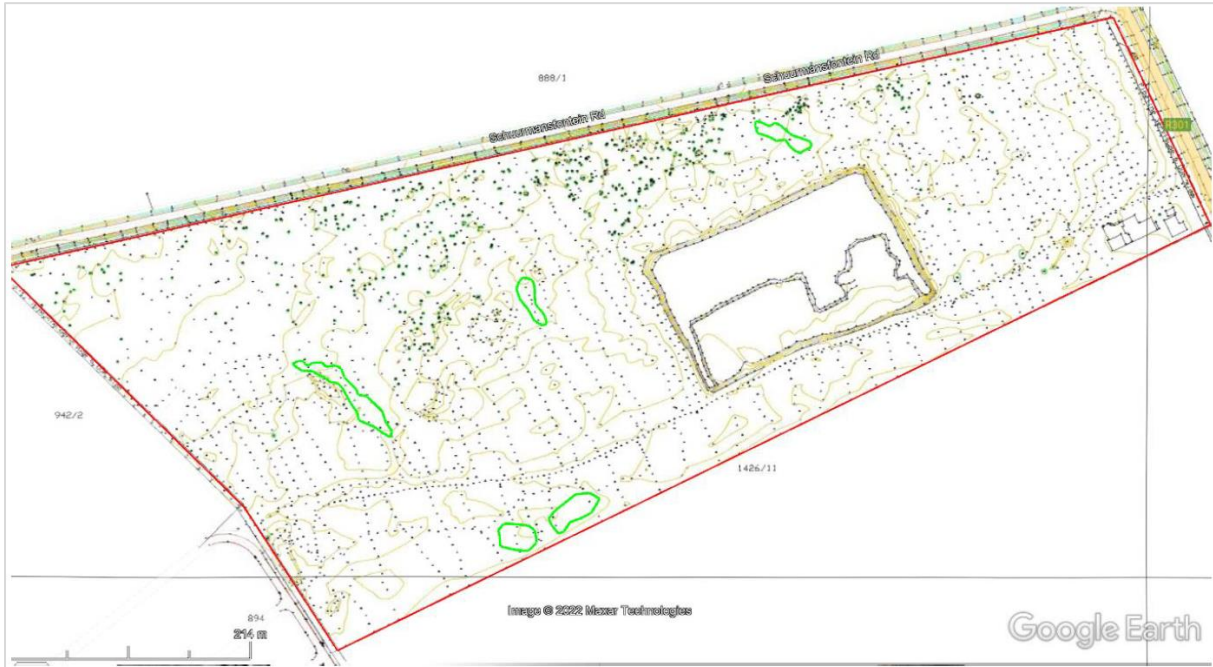
Figure 25: Topographical survey of the site, overlaid in Google Earth with the delineated wetland areas shown.
